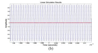
Fig. 7. Steady state of Tesla transformer excited with square wave in resonance: (a) general response and (b) zoomed.
