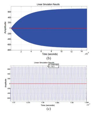
Fig. 8. Resonant response of Tesla transformer to sinusoidal excitation: (a) transient response, (b) general response, and (c) zoomed response of steady state.
