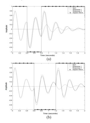
Fig. 5. Response of Tesla transformers to square wave at rise and fall: (a) sum and (b) subtraction.
