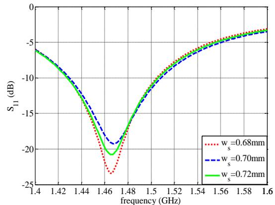
Fig. 6. Simulated  $S_{11}$  with different coupling slot widths.
