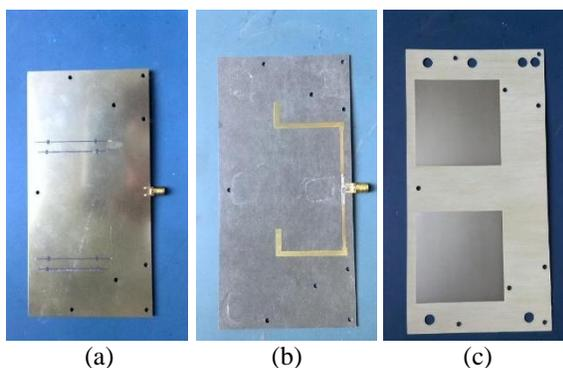
Fig. 11. Antenna prototype: (a) the ground plane with coupling slots, (b) the feed network, and (c) the radiating patches.
