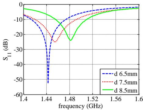
Fig. 8. Simulated  $S_{11}$  with different tiny slot positions.
