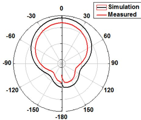
Fig. 9. H-plane pattern of the proposed antenna.
