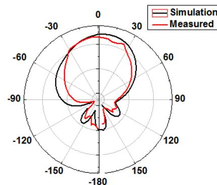
Fig. 8. E-plane pattern of the proposed antenna.
