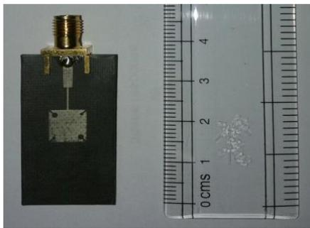
Fig. 6. Fabricated circularly polarized asymmetric slit patch antenna.
