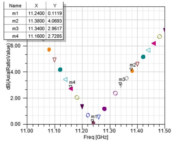
Fig. 3. Axial ratio of the proposed antenna.
