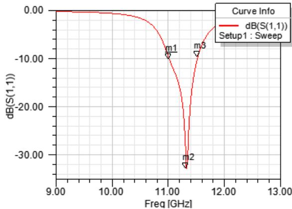
Fig. 2. Reflection coefficient (S<sub>11</sub>) of the proposed antenna.
