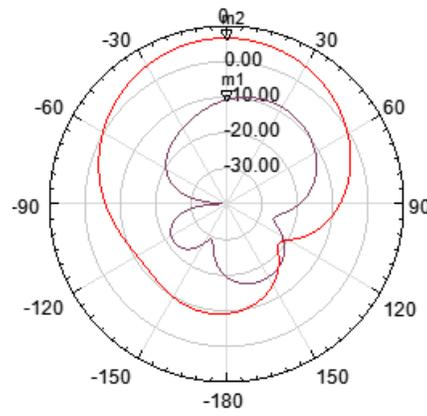
Fig. 4. Radiation pattern of the proposed antenna.
