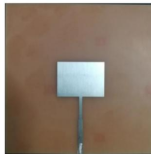
Fig. 5. Prototype of patch antenna (top view).
