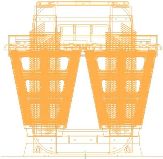
Fig. 3. The mechanical design of the pulse transformer.
