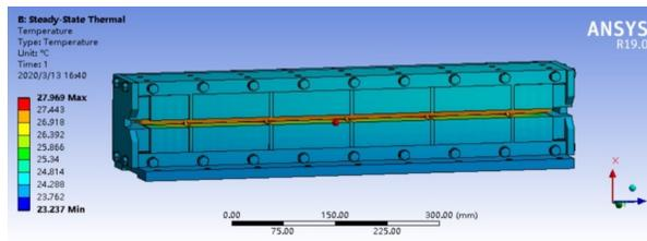
Fig. 6. Internal temperature distribution of the septum.
