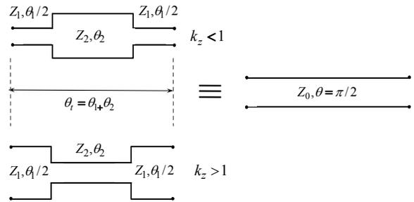
Fig. 1. The step impedance transmission line configuration (SITL).
