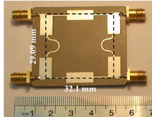
Fig. 4. The photo of the fabricated coupler.
