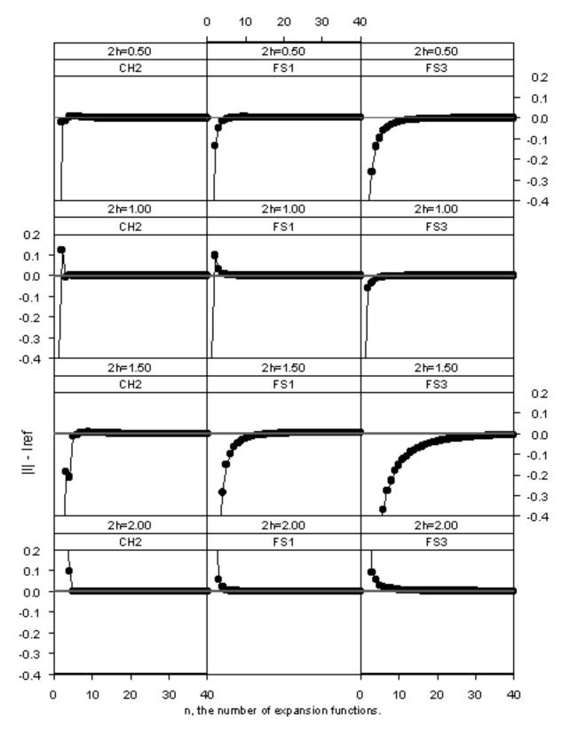
Figure 2b. Plots of (||- Iref) at the center of each dipole excited by a plane wave for each of the three main expansion functions.
