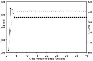
Figure 1b. Plots of the components of the current on a perfectly conducting cylinder illuminated by a TM wave.
