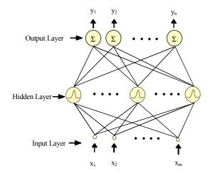
Figure 3. Radial basis function network.
