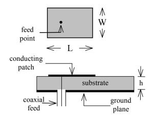
Figure 1. Geometry of rectangular microstrip antenna.
