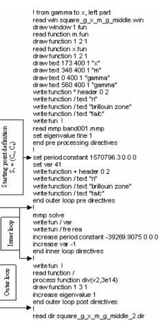
Fig. 10: The algorithm for band diagram computation written in the MaX-1 script language.
