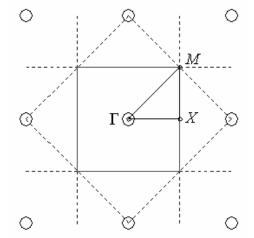
Fig. 2: Construction of the 1<sup>st</sup> Brillouin zone (solid square), its irreducible part (triangle  $\Gamma$ -X-M) and characteristic points for band structure computation ( $\Gamma$ , X, and M).
