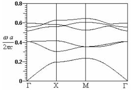
Fig. 12: The band diagram of the photonic crystal with dielectric rods and square lattice, E-polarization, the first 6 modes.
