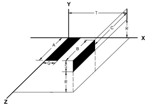
Figure 5. Two tapes of negligible thickness, whose axis are parallel and widths are perpendicular. The current is in the  $z$ -direction.
