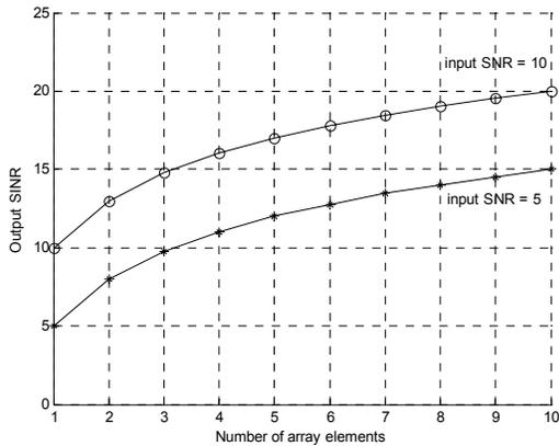
Fig. 4. Improvement of output  $SINR$  using adaptive antenna arrays.
