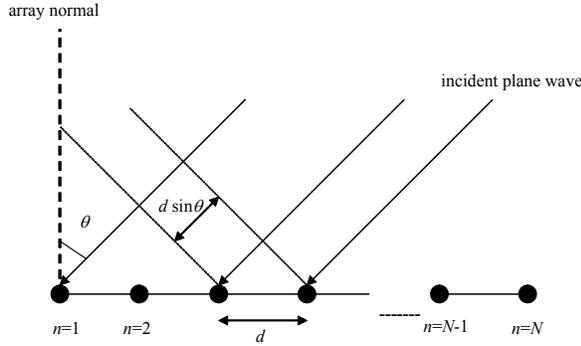
Fig. 5. Equispaced linear array of  $N$  sensors.
