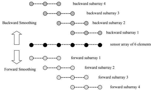
Fig. 13. FBSS applied to a six-element sensor array.
