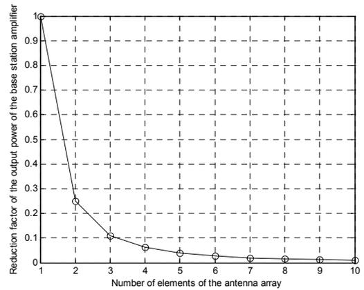
Fig. 3. Reduction in transmission power at the base station using adaptive antenna arrays.
