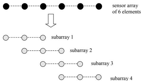
Fig. 12. FSS applied to a six-element sensor array.
