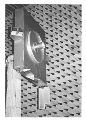
Fig. 5. Real mock-up of the Stentor satellite incide the CNES anechoic chamber.
