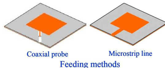
Fig. 2. Patch shapes and two common feeding methods.
