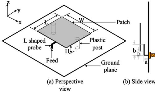
Fig. 5. Geometry of the L-probe coupled patch antenna.
