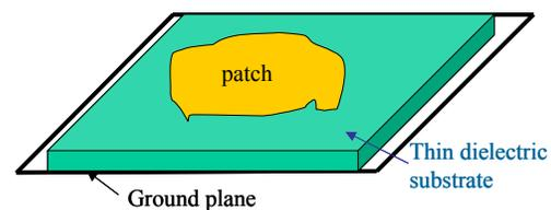
Fig. 1. Basic structure of a microstrip patch antenna.
