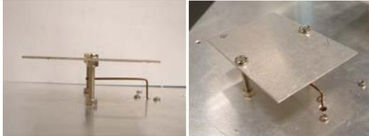
Fig. 6. Prototype of the L-probe coupled patch antenna.
