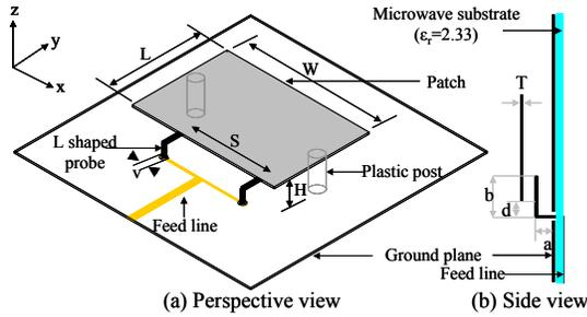
Fig. 9. Geometry of the twin-L-probe fed patch antenna.
