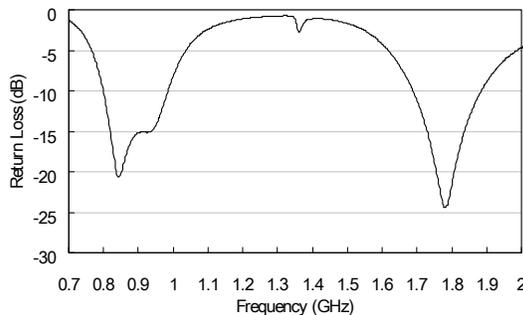
Fig. 17. Simulated return loss of the antenna shown in Figure 16 with the following dimensions:  $L_1 = W_1 = 102$  mm ( $0.324\lambda_1$ ),  $H_1 = 45.5$  mm ( $0.145\lambda_1$ ),  $b_1 = 51$  mm ( $0.162\lambda_1$ ),  $a_1 = 31$  mm ( $0.098\lambda_1$ ),  $S_1 = 4$  mm ( $0.0127\lambda_1$ ),  $g_1 = 2$  mm ( $0.0064\lambda_1$ ),  $g_2 = 90$  mm ( $0.286\lambda_1$ ),  $c_2 = 25.5$
