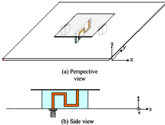
Fig. 20. Geometry of the printed meandering strip fed patch antenna.
