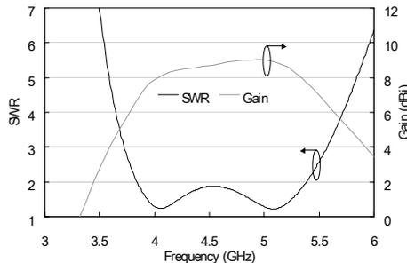
Fig. 7. Simulated SWR and gain versus frequency of the L-probe coupled antenna of Figure 6 with the following dimensions:  $W=30$  mm,  $L=25$  mm,  $H=6.6$  mm,  $a=5.5$  mm,  $b=10.5$  mm,  $d=2$  mm.
