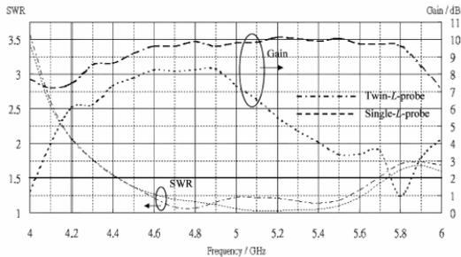
Fig. 10. Measured SWR and gain of the twin-L-probe coupled patch of Figure 9 with the following dimensions:  $L=22$  ( $0.367\lambda$ ),  $H=6$  ( $0.1\lambda$ ),  $W=44$  ( $0.733\lambda$ ),  $T=0.3$  ( $0.005\lambda$ ),  $a=4.5$  ( $0.075\lambda$ ),  $b=12$  ( $0.2\lambda$ ),  $v=2$  ( $0.033\lambda$ ),  $d=0$  ( $0\lambda$ ),  $s=28.6$  ( $0.477\lambda$ ). The case of single L-probe coupled patch is also shown for comparison. (From Mak et. al. [9], c 2005 IEEE)
