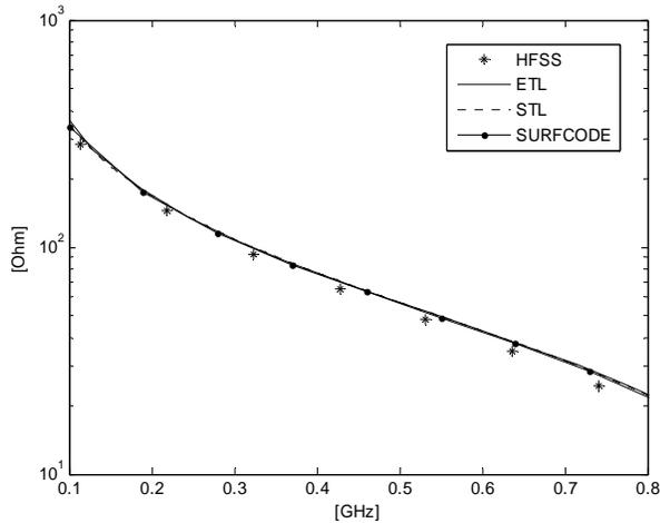
Fig. 3. Low frequency behaviour of the absolute value of the input impedance, Case 1.
