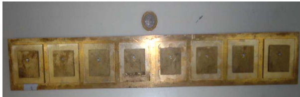
Fig. 5. Antenna array ( w_x = w_y = 72\text{ mm} , f = 2.45\text{ GHz} , \Delta x = 0.5\lambda , N = 8 and h = 6\text{mm} ).
