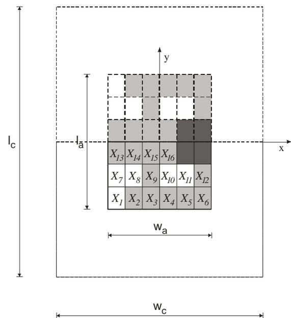
Fig. 1. Top view of cavity and patch.
