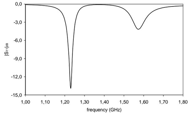
Fig. 4. Return loss of the optimal patch.
