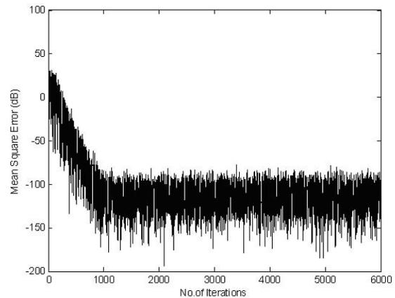
Fig. 7. Mean square error vs. number of iterations for SMI-initialized LMMN algorithm ( $N = 4$ ,  $d = 0.5\lambda$ ,  $SNR = 10$  dB,  $SIR = -10$  dB,  $\mu = 1 \times 10^{-3}$ ,  $\delta = 0.40$ ,  $\theta_S = 20^\circ$ ,  $\theta_I = -40^\circ$ ).
