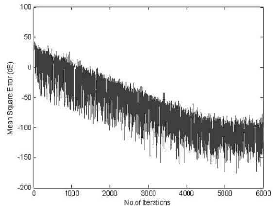
Fig. 6. Mean square error vs. number of iterations for LMS algorithm ( $N = 4$ ,  $d = 0.5\lambda$ ,  $SNR = 10$  dB,  $SIR = -10$ dB,  $\mu = 1 \times 10^{-3}$ ,  $\theta_S = 20^\circ$ ,  $\theta_I = -40^\circ$ ).
