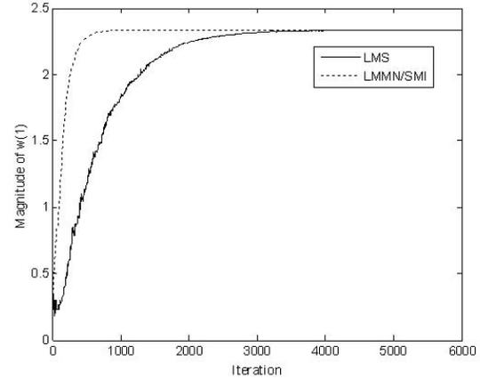
Fig. 5. Convergence of  $\mathbf{w}(1)$  using both LMS and SMI-initialized LMMN algorithm ( $N = 4$ ,  $d = 0.5\lambda$ ,  $SNR = 10$  dB,  $SIR = -10$ dB,  $\mu = 1 \times 10^{-3}$ ,  $\delta = 0.40$ ,  $\theta_S = 0^\circ$ ,  $\theta_I = -60^\circ$ ).
