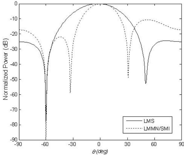
Fig. 4. Output beampattern using LMS and proposed LMMN/SMI algorithm ( $N = 4$ ,  $d = 0.5\lambda$ ,  $SNR = 10$  dB,  $SIR = -10$ dB,  $\mu = 1 \times 10^{-3}$ ,  $\delta = 0.40$ ,  $\theta_S = 0^\circ$ ,  $\theta_I = -60^\circ$ ).
