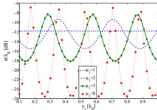
Fig. 9. Normalized RCS of the crack with  $w = 0.2 \lambda_0$ ,  $b = 0.2 \lambda_0$ ,  $\epsilon_r = 2.7 + 0.03i$ ,  $\mu_r = 1$  versus paint thickness for different permeabilities.
