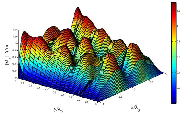
Fig. 3. Distribution of magnetic current density in the crack computed by the KP method for crack of case b.
