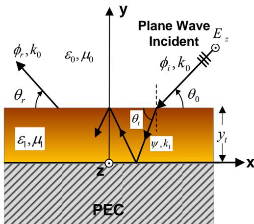
Fig. A. Geometry of a dielectric slab on an infinite ground plane.
