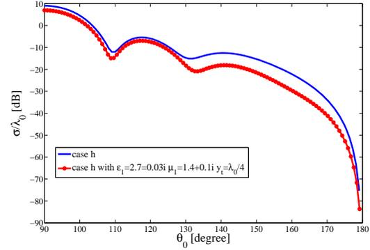
Fig. 7. Normalized backscattering RCS of the narrow crack of case h and this case with a  $\lambda_0 / 4$  dielectric layer of  $\epsilon_1 = 2.7 + 0.03i$  and  $\mu_1 = 1.4 + 0.1i$ .
