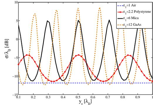
Fig. 8. Normalized RCS of the crack with  $w = 0.2 \lambda_0$ ,  $b = 0.2 \lambda_0$  as a function of coating thickness for different permittivities.
