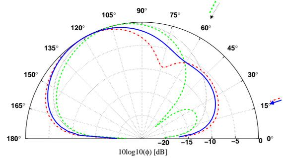
Fig. 11. Scattering far-field pattern for a crack where  $w = b$ ,  $2ka = 5$ ,  $y_t = \lambda_0 / 7$ , and dielectric filled material characteristics are depicted in the figure legend
