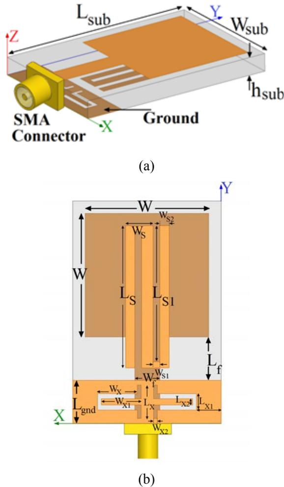
Fig. 1. Geometry of the proposed square monopole antenna; (a) bottom view and (b) side view.
