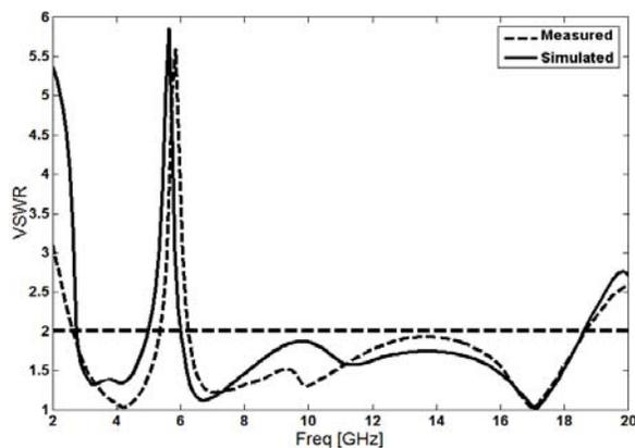
Fig. 8. Measured and simulated VSWR for the proposed antenna.
