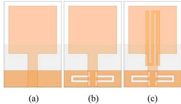
Fig. 2. (a) The ordinary square monopole antenna, (b) antenna with a pair of rotated  $\Omega$ -shaped slots in the ground plane, and (c) the proposed square monopole antenna.
