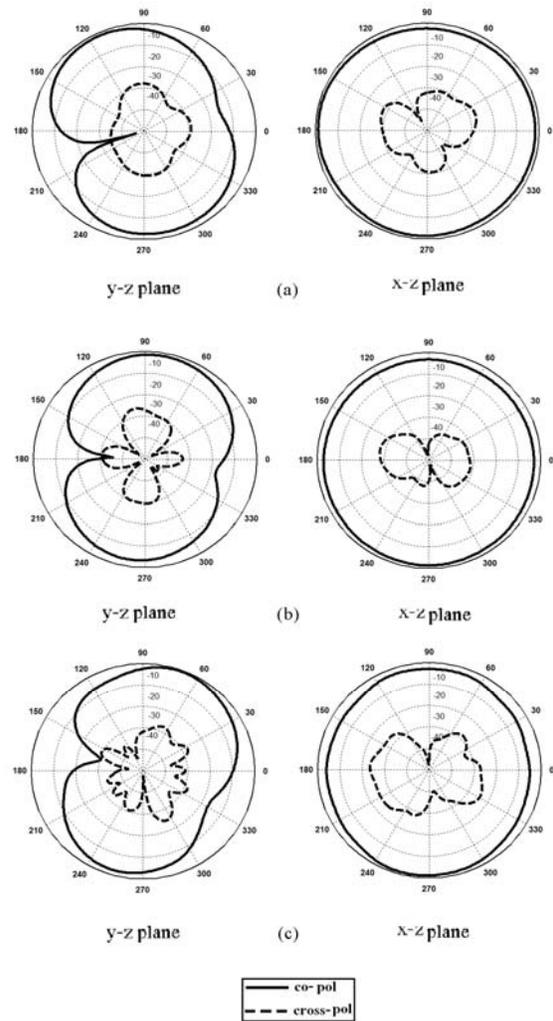
Fig. 9. Measured radiation patterns of the proposed antenna at (a) 4 GHz, (b) 7 GHz, and (c) 10 GHz.
