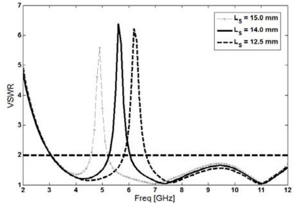
Fig. 5. Simulated VSWR characteristics for the proposed antenna with different values of  $L_S$ .
