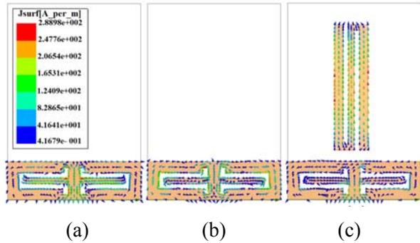
Fig. 4. Simulated surface current distributions on the ground plane for (a) the square antenna with a pair of  $\Omega$ -shaped slots in the ground plane at a third resonance frequency (11.2 GHz), (b) at fourth resonance frequency (17.1 GHz), and (c) for the proposed antenna at the notch frequency (5.5 GHz).
