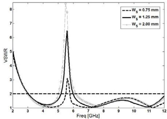
Fig. 6. Simulated VSWR characteristics for the proposed antenna with different values of  $W_S$ .
