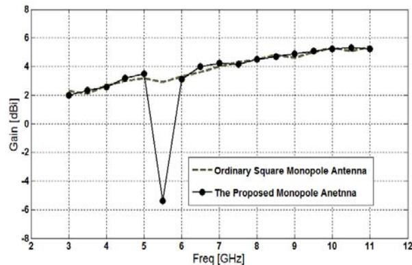
Fig. 10. Maximum gain comparisons for the ordinary monopole antenna (simulated), and the proposed antenna (measured) in the z-axis direction (x-z plane).
