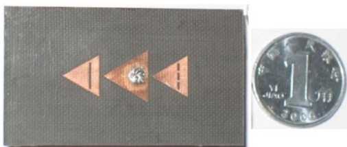
Fig. 3. Fabricated antenna model (mode DN).
