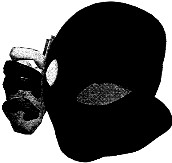
Figure 14: MoM model of IEEE generic head, hand and generic phone at 1800MHz. Peak-SAR-Contiguous 10g volume is also shown.
