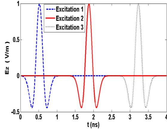
Fig. 7. Second-order Gaussian pulses with different time delays.
