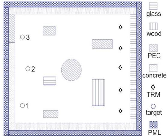
Fig. 2. Simplified 2D lossless indoor space model.
