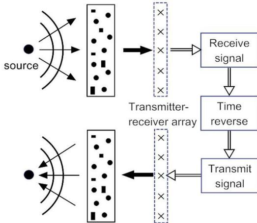
Fig. 1. Typical process of TR.
