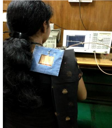
Fig. 5. Return loss measurement for antenna placed on-body.
