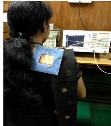
Fig. 5. Return loss measurement for antenna placed on-body.
