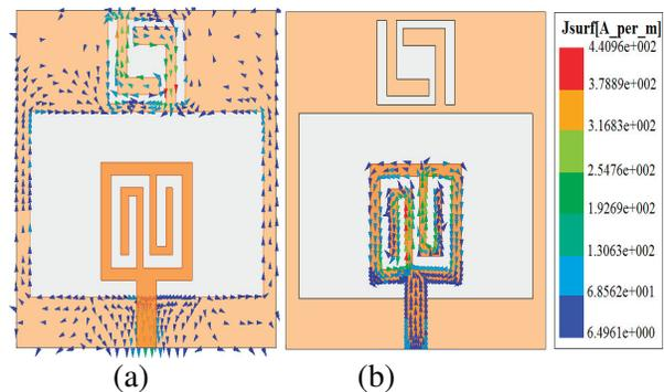
Fig. 4. Simulated surface current distributions for the proposed antenna at, (a) 9 GHz (resonance frequency) and (b) 5.5 GHz (notched frequency).
