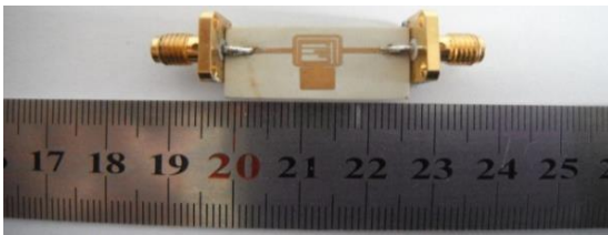
Fig. 16. Prototype of the proposed multi-notch band UWB filter.
