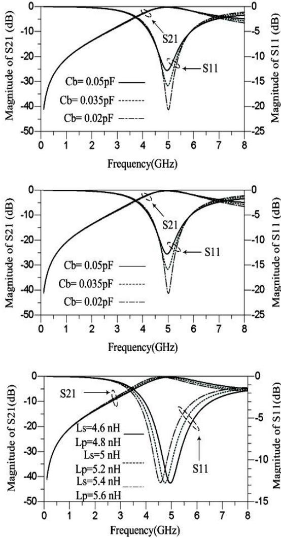
Fig. 7. Simulated results of the half-resonator model.
