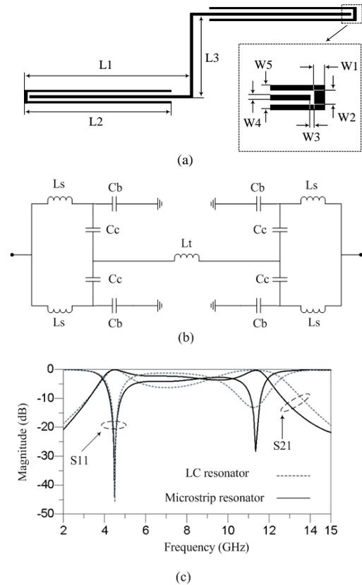
Fig. 1. Basic resonator: (a) layout, (b) LC model, and (c) frequency responses.
