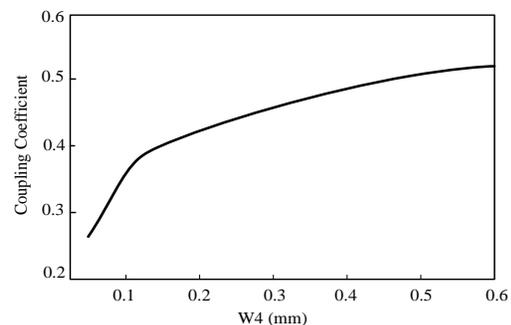
Fig. 4. Coupling coefficient of the proposed resonator versus the width of the central line.
