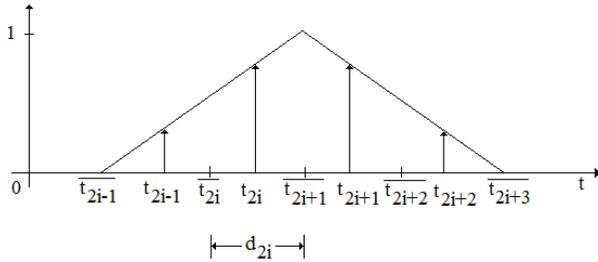
Fig. 5. Triangle function  $T(t - \bar{t}_{2i+1})$  and four impulse approximation.
