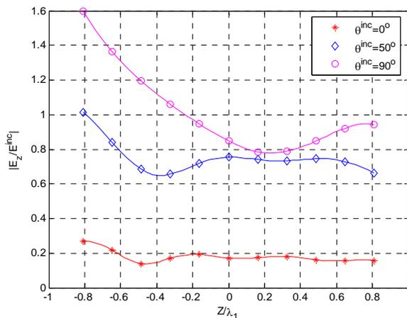
Fig. 12. Fields on the  $z$ -axis of a Von Karman radome for  $\theta^{inc} = 0^\circ, 50^\circ, \text{ and } 90^\circ$ .
