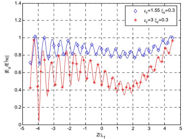
Fig. 9. Fields on the  $z$ -axis of a cylindrical radome for  $\theta^{inc} = 0^\circ$ .
