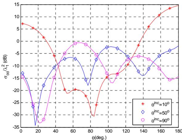
Fig. 13.  $\sigma_{\theta\theta}$  of a Von Karman radome for  $\theta^{inc} = 0^\circ, 50^\circ, \text{ and } 90^\circ$ .
