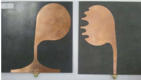
Fig. 2. Photograph of fabricated ATSAs.
