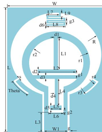
Fig. 1. Geometry of the proposed antenna.
