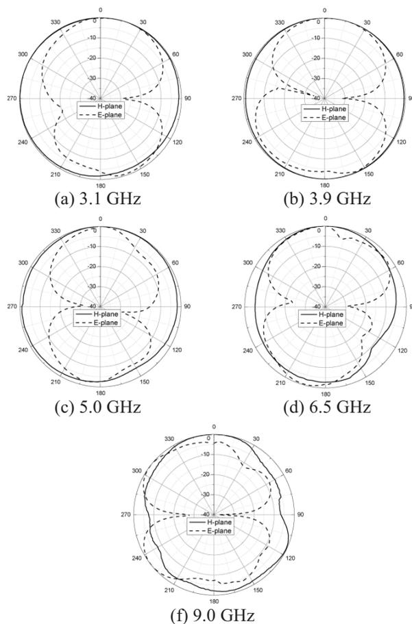
Fig. 6. Radiation patterns of the proposed antenna.
