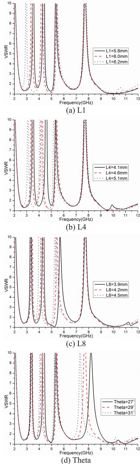
Fig. 2. Parameter effects on the band-notched characteristics of the proposed antenna.
