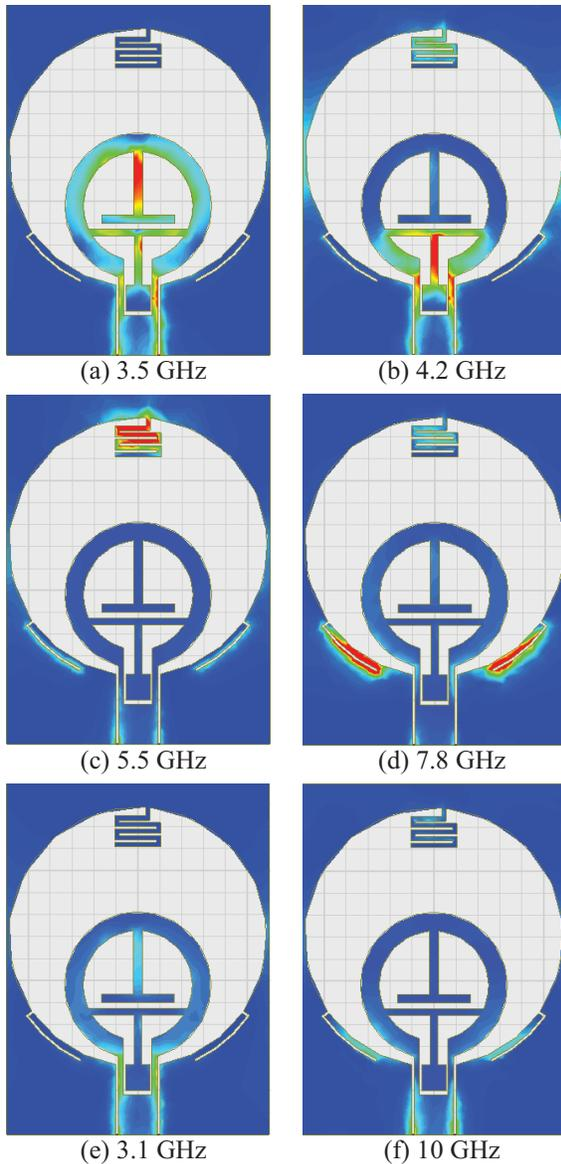
Fig. 3. Current distribution of the proposed antenna.
