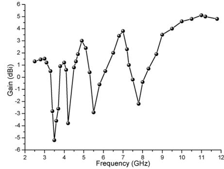
Fig. 7. Gains of the proposed antenna.
