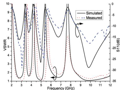
Fig. 5. Measured VSWR and  $S_{11}$  of the antenna.
