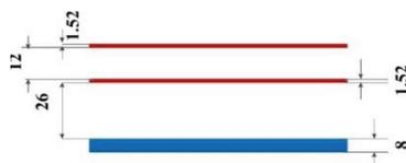
Fig. 2. Distances and thicknesses of antenna layers in mm.
