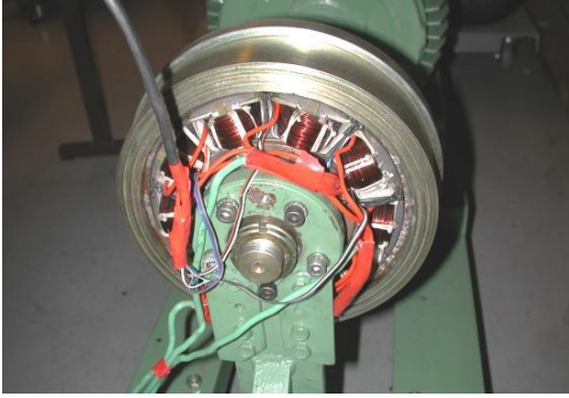
Fig. 1. Prototype of the wheel motor. The inner stator is visible with the coils rolled up around the teeth [9].
