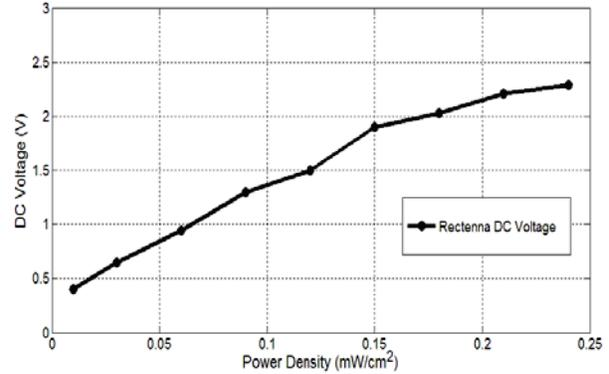
Fig. 9. Measured DC voltages against power density.
