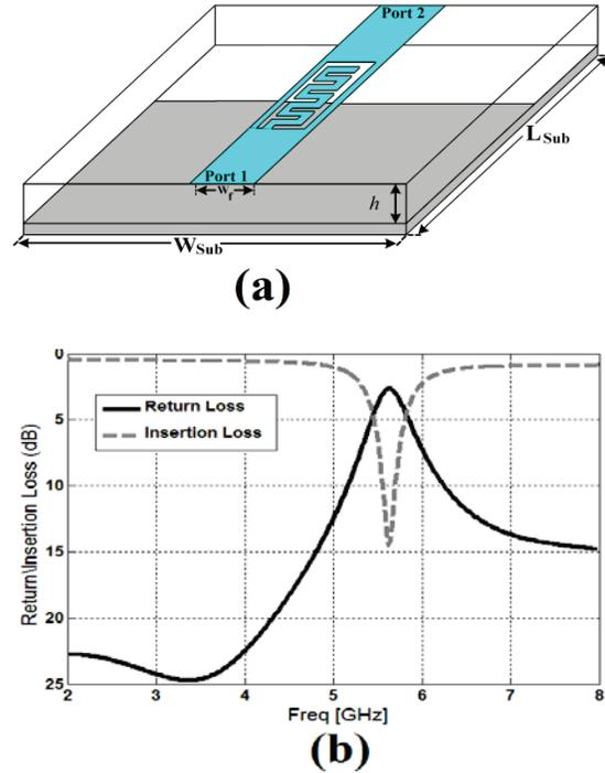
Fig. 3. (a) Geometry of the proposed Defected Microstrip Structure (DMS), and (b) simulated return/insertion loss characteristics for the proposed defected microstrip structure.
