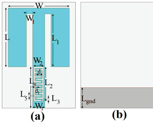
Fig. 2. Geometry of proposed microstrip-fed monopole antenna: (a) top view, and (b) bottom view.
