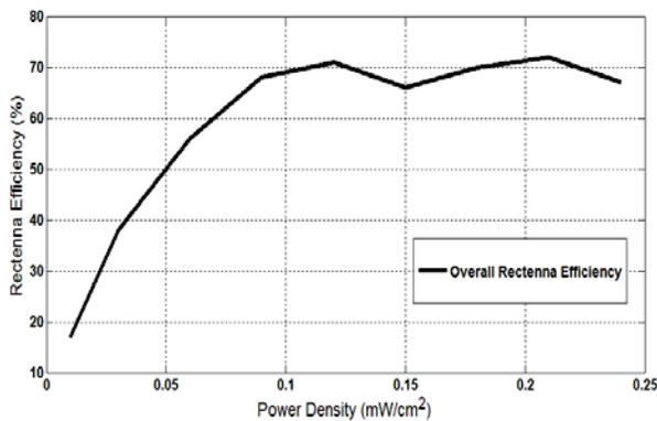
Fig. 8. Measured rectenna efficiency against power density.
