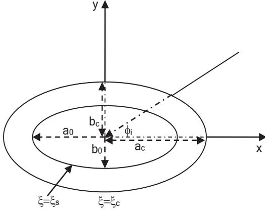
Fig. 1. Geometry of the chiral coated PEMC elliptic cylinder.
