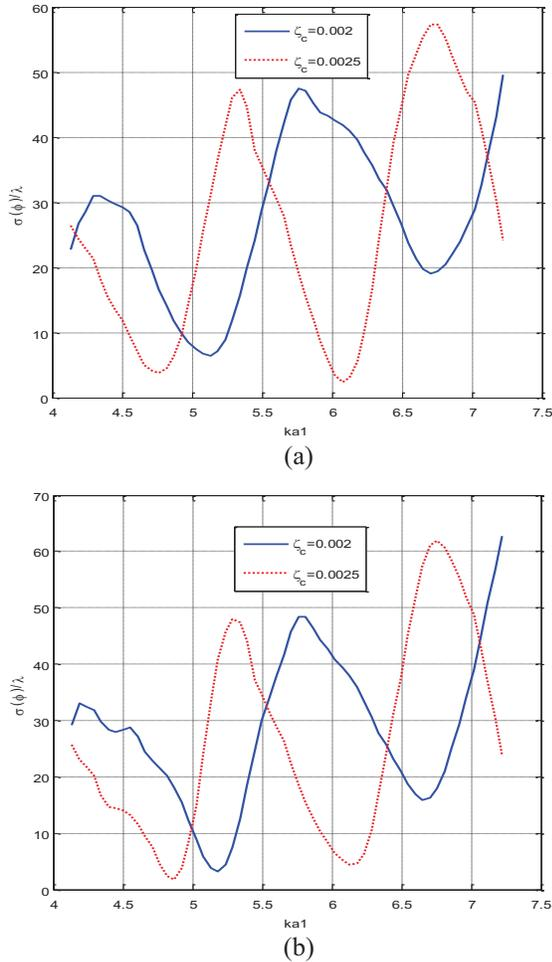
Fig. 6. Normalized bistatic width versus  $ka_1$  for PEMC elliptic cylinders of different admittances coated with  $\epsilon_{rc}=3.0$ ,  $\mu_{rc}=1.0$ ,  $\phi_i=0.0^\circ$ ,  $a=0.4\lambda$ ,  $b=0.2\lambda$ : (a)  $\nu=45^\circ$ , and (b)  $\nu=75^\circ$ .
