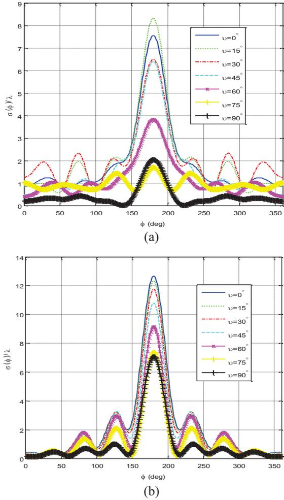
Fig. 3. Normalized bistatic width versus scattering angle for PEMC elliptic cylinders of different admittances coated with  $\epsilon_{rc}=2.5$ ,  $\mu_{rc}=1.0$ ,  $\phi_i=0^\circ$ : (a)  $\zeta_c=0.002$ , and (b)  $\zeta_c=0.0015$ .
