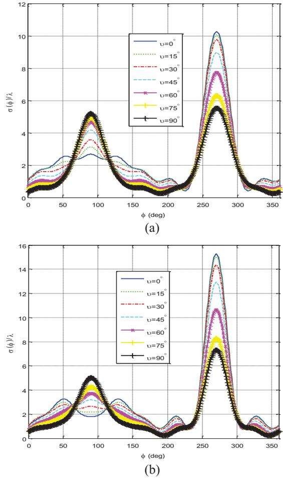
Fig. 4. Normalized bistatic width versus scattering angle for PEMC elliptic cylinders of different admittances coated with  $\epsilon_{rc}=2.5$ ,  $\mu_{rc}=1.0$ ,  $\phi_i=90^\circ$ : (a)  $\zeta_c=0.002$ , and (b)  $\zeta_c=0.0015$ .
