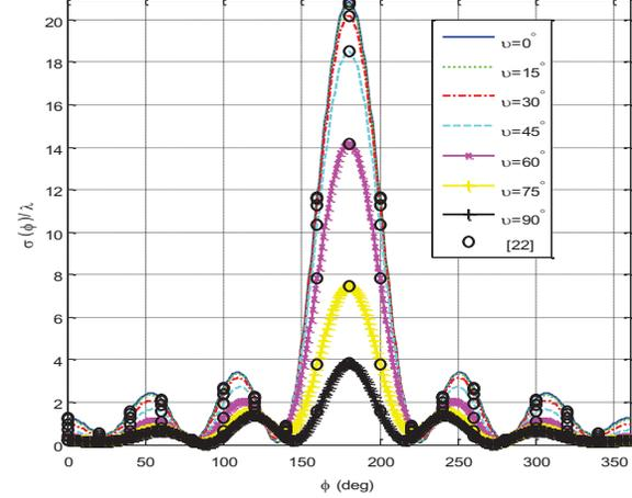
Fig. 2. Normalized bistatic width versus scattering angle for PEMC elliptic cylinders of different admittances coated with  $\epsilon_{rc}=2.5$ ,  $\mu_{rc}=1.0$ ,  $\phi_i=0^\circ$ , and  $\zeta_c=0.0$ .
