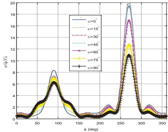
Fig. 5. Normalized bistatic width versus scattering angle for PEMC elliptic cylinders of different admittances coated with  $\epsilon_{rc}=3.0$ ,  $\mu_{rc}=1.0$ ,  $\phi_i=90^\circ$  and  $\zeta_c=0.002$ .
