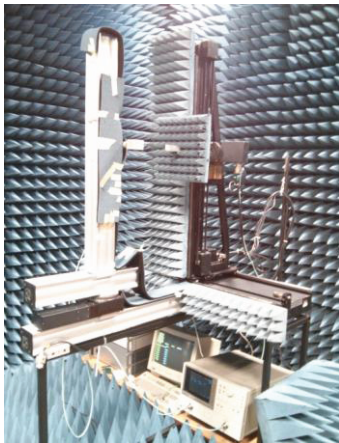
Fig. 6. Planar near-field range: the antenna backed with pyramidal absorbers is the open-ended waveguide probe. The other antenna is the covered monopole-like slot antenna under test. Absorbers have been taped on the tower that holds the antenna under test.
