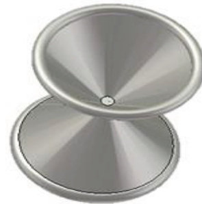
Fig. 1. Antenna structure - biconical antenna with ring.
