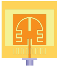
Fig. 7. Geometry of the proposed antenna.
