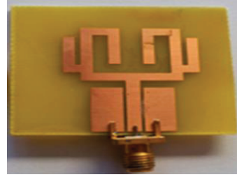
Fig. 7. Photograph of the fabricated compact tri-band antenna.
