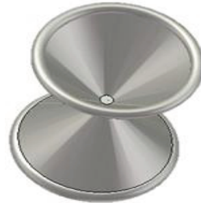
Fig. 1. Antenna structure - biconical antenna with ring.
