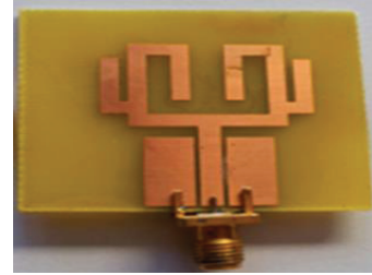
Fig. 7. Photograph of the fabricated compact tri-band antenna.
