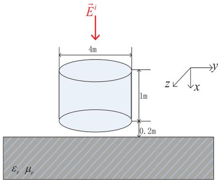
Fig. 3. The cylinder model in half space.
