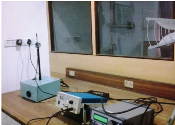
Fig. 9. Experimental set-up for radiation pattern measurement.
