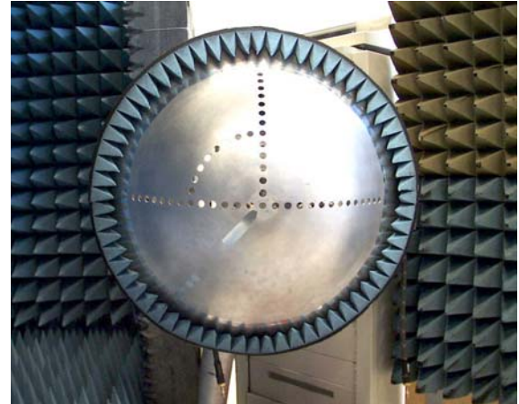
Figure 14. The geometry of the experimental doubly curved antenna. Courtesy of Ericsson Microwave Systems AB.
