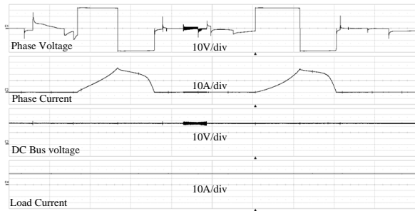
(a) Case a: i_{max} = 40 A, \theta_{on} = -7.8^\circ , \theta_{off} = 5.5^\circ , I_L = 16.1 A, and u = 36.2 V
