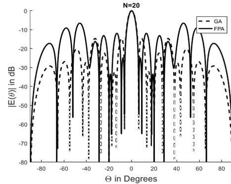
Fig. 3. Radiation pattern with null  $20^\circ$ .
