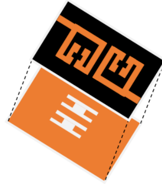
Fig. 4. 3-D model of the proposed dual-band bandpass filter.
