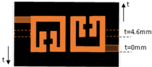
Fig. 7. 2-D layout of the proposed dual-band bandpass filter at different value of (t).
