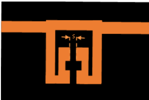
Fig. 1. The 2-D layout of the double microstrip ring resonator.
