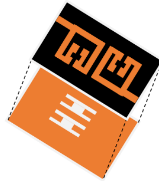
Fig. 4. 3-D model of the proposed dual-band bandpass filter.
