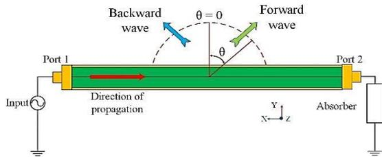
Fig. 1. The measurement, obtaining scenario for the radiation angle of the main lobe. Showing side view of the antenna including the SMA connectors.
