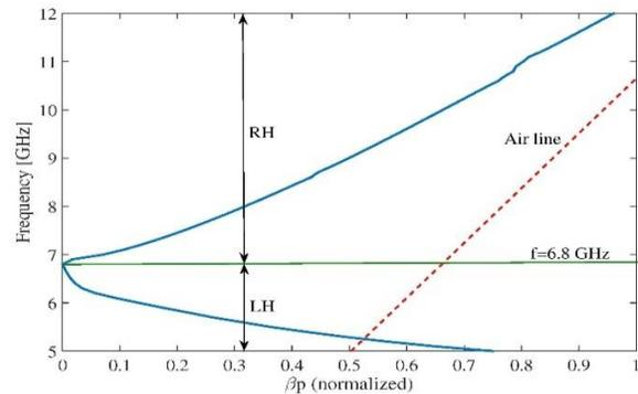
Fig. 5. Dispersion diagram of proposed the unit-cell.
