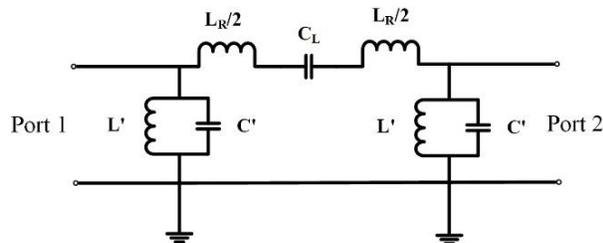
Fig. 4. Equivalent circuit model for the proposed unit-cell.
