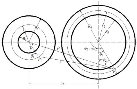
Fig. 2. Plan view of two coplanar disk coils.
