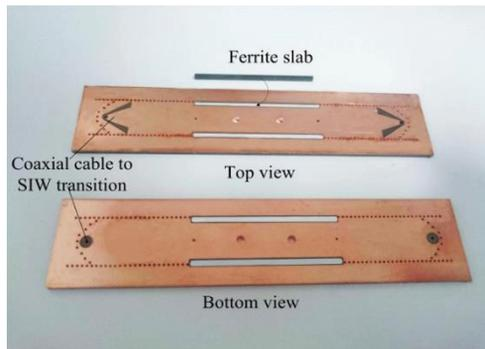
Fig. 7. Photograph of the fabricated ferrite-loaded SIW frequency-agile bandpass filter.
