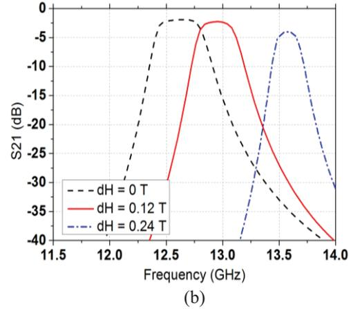
Fig. 8. Simulated S-parameter of the designed filter with different internal magnetic bias,  $dH$ . (a) Return loss and (b) insertion loss.
