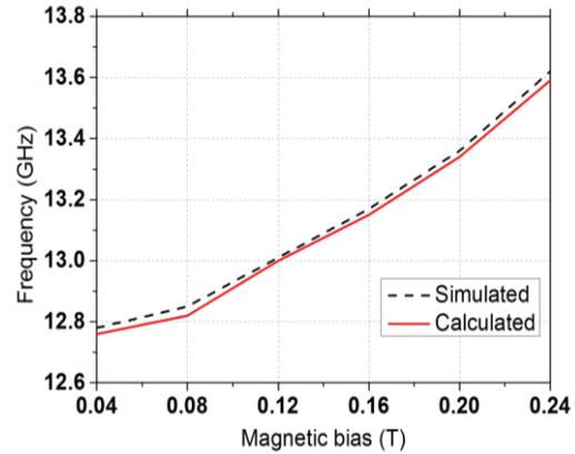
Fig. 6. Operating frequency of the bandpass filter versus DC magnetic bias.
