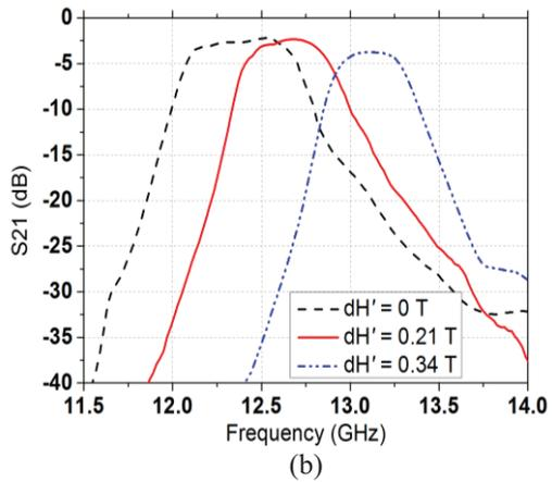
Fig. 9. Measured S-parameter with different total applied external magnetic bias,  $dH'$ . (a) Return loss and (b) insertion loss.
