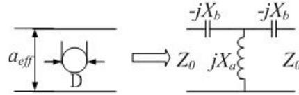
Fig. 5. Metalized post in a waveguide and its equivalent circuit.
