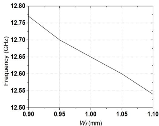
Fig. 11. Tolerance of the width of the ferrite slabs  $W_f$ .
