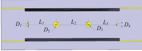
Fig. 4. Configuration of the proposed three-order frequency-agile filter.
